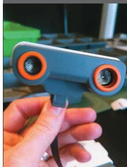
Fig. 5 The ultrasonic sensor serves as the eyes of the robot.
